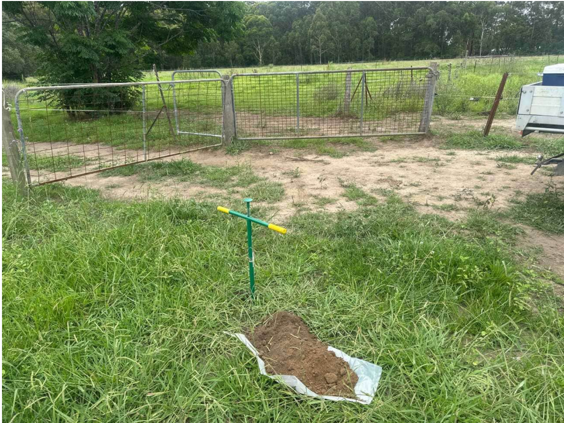
Photograph 19: Boreholes advanced by handauger – location HA205 (3 December 2024).
