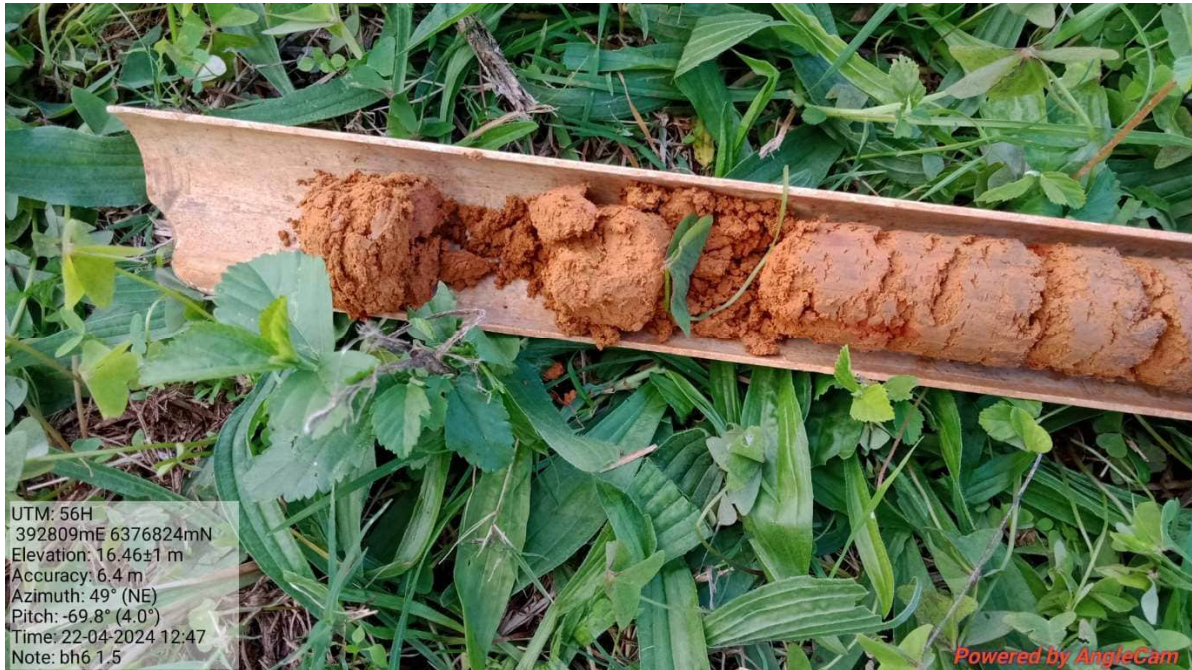
Photograph 5: Location BH06. Natural red, silty clay at 1.5 m BGL, representative of natural sub-soil clay across the investigation area (22 April 2024).
