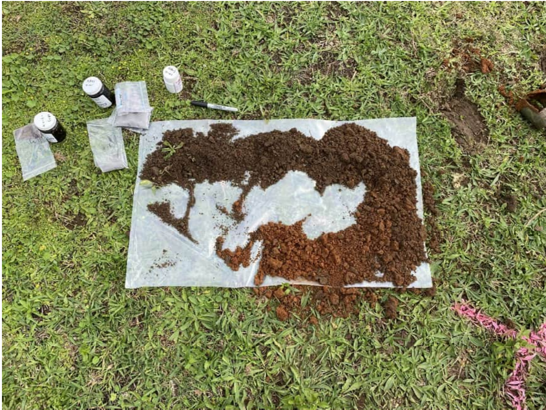
Photograph 3: Hand auger location HA03 showing dark brown clay topsoil, representative of near surface material across the investigation area (22 April 2024).
