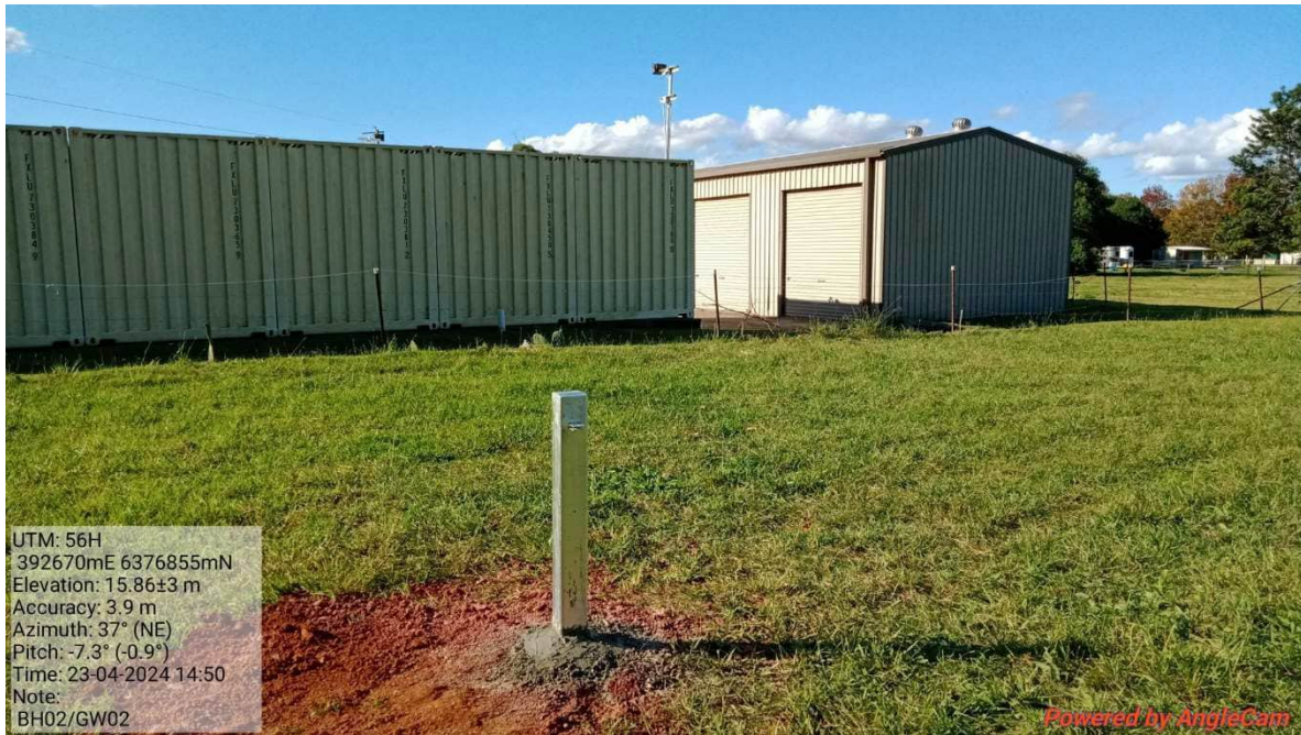
Photograph 11: Groundwater well GW02 post installation (23 April 2024).
