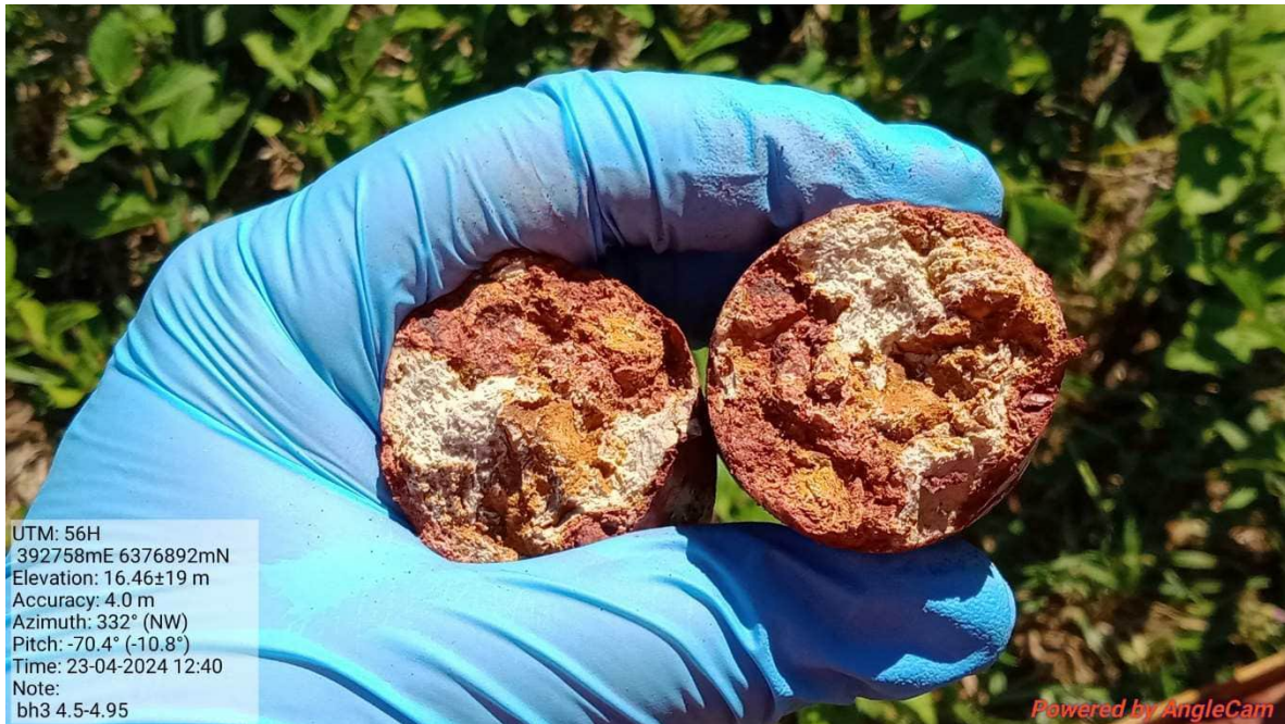
Photograph 9: Location BH03/GW03. Mottled red, brown and light grey clay at approximately 4.5 mBGL (23 April 2024).
