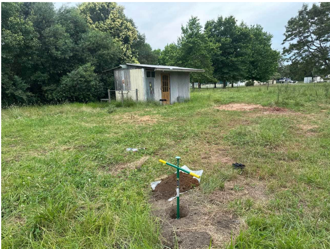
Photograph 18: Boreholes advanced by handauger – location HA204 (3 December 2024).
