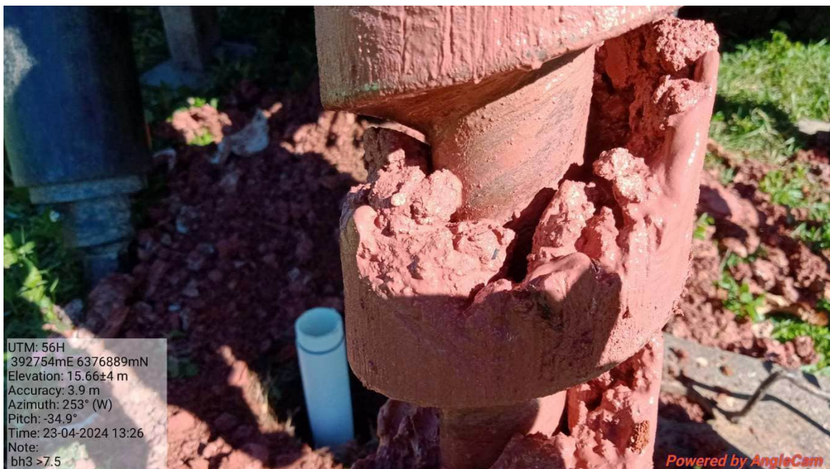
Photograph 10: Location BH03/GW03. Saturated clay material encountered from 7.0 mBGL (23 April 2024).
