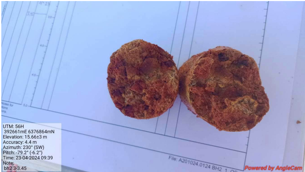
Photograph 7: Location BH062/ GW02. Dark red ironstone gravels noted within natural clay from approximately 3.0 m BGL (23 April 2024).
